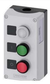
ENCLOSURE FOR COMMAND DEVICES, 22MM, ROUND, ENCLOSURE MATERIAL PLASTIC, ENCLOSURE TOP PART GRAY, 3 COMMAND POINTS PLASTIC, C=INDICATOR LIGHT CLEAR, LABEL LED 24V, SCREW TERMINAL, B=PUSHBUTTON GREEN, LABEL: I, 1NO, SCREW TERMINAL, A=PUSHBUTTON RED, LABEL: O, 1NC, SCREW TERMINAL, BASE MOUNTING, TOP AND BOTTOM 1 X M20 EACH
